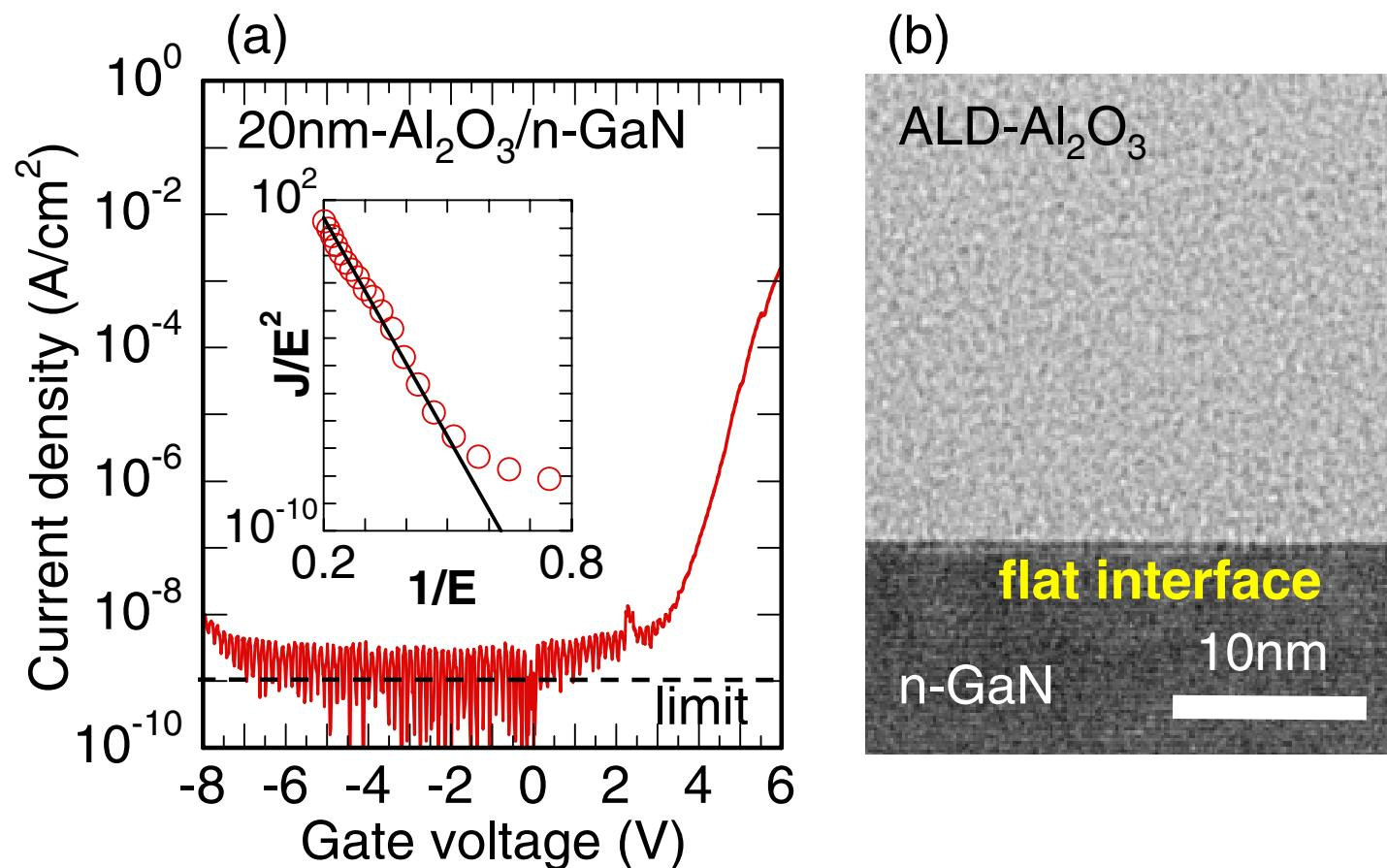
An amorphous phase was kept in the atomic bonds of  $\text{Al}_2\text{O}_3$ .
