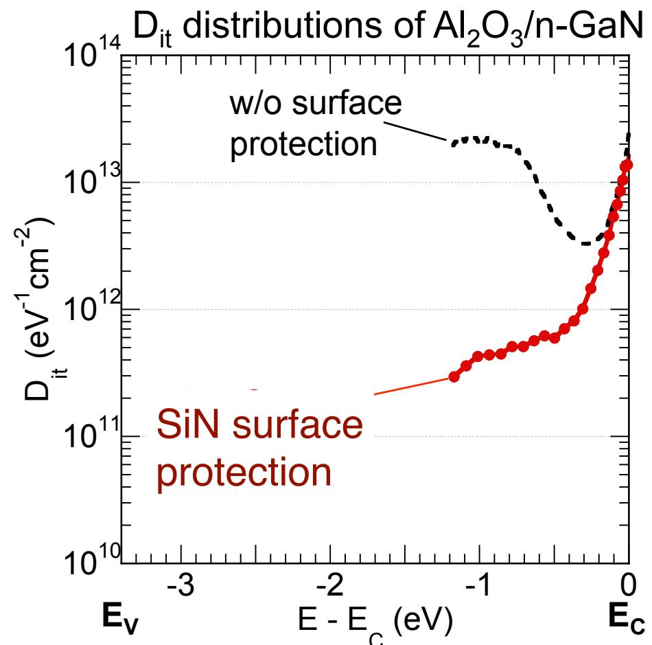
The surface protection layer could suppress N desorption and related chemical disorder at the GaN surface.
