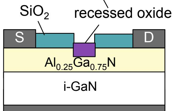
Selective formation of recessed oxide between source and drain electrode was achieved.
