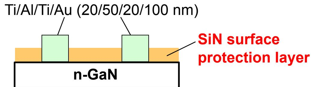
3. Ohmic-annealing (800°C, 1 min, N<sub>2</sub> ambient)
