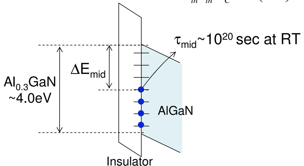
Large bandgap of AlGaN causes extremely long time for electron emission from the interface states near midgap or at deeper energies.
