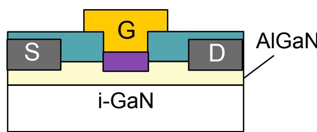
➤ A plan-view optical microscope image and cross-sectional illustration of recessed oxide gate HEMT
