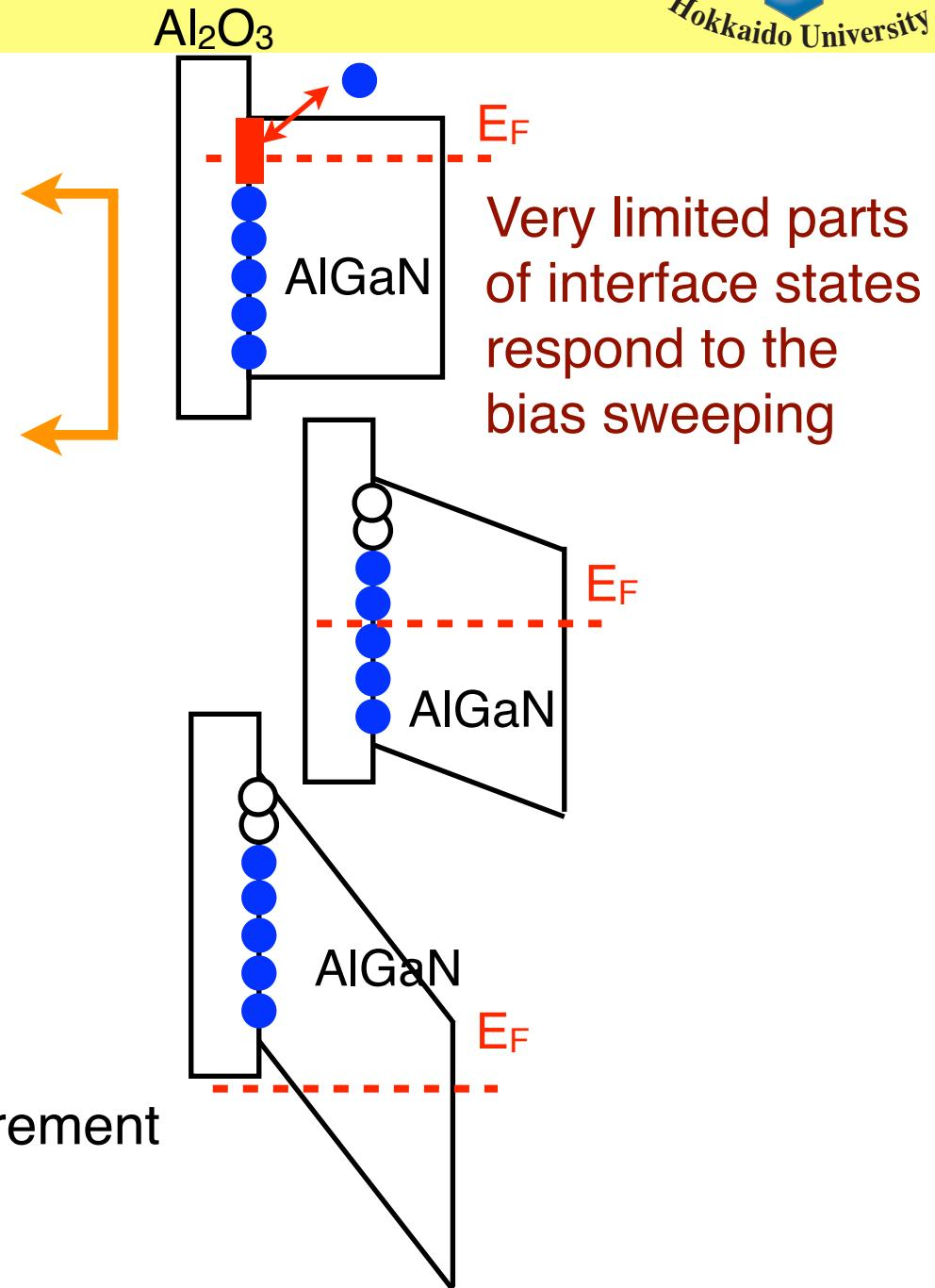
Almost all of interface states are in “sleeping” condition during C-V measurement at room temperature.
