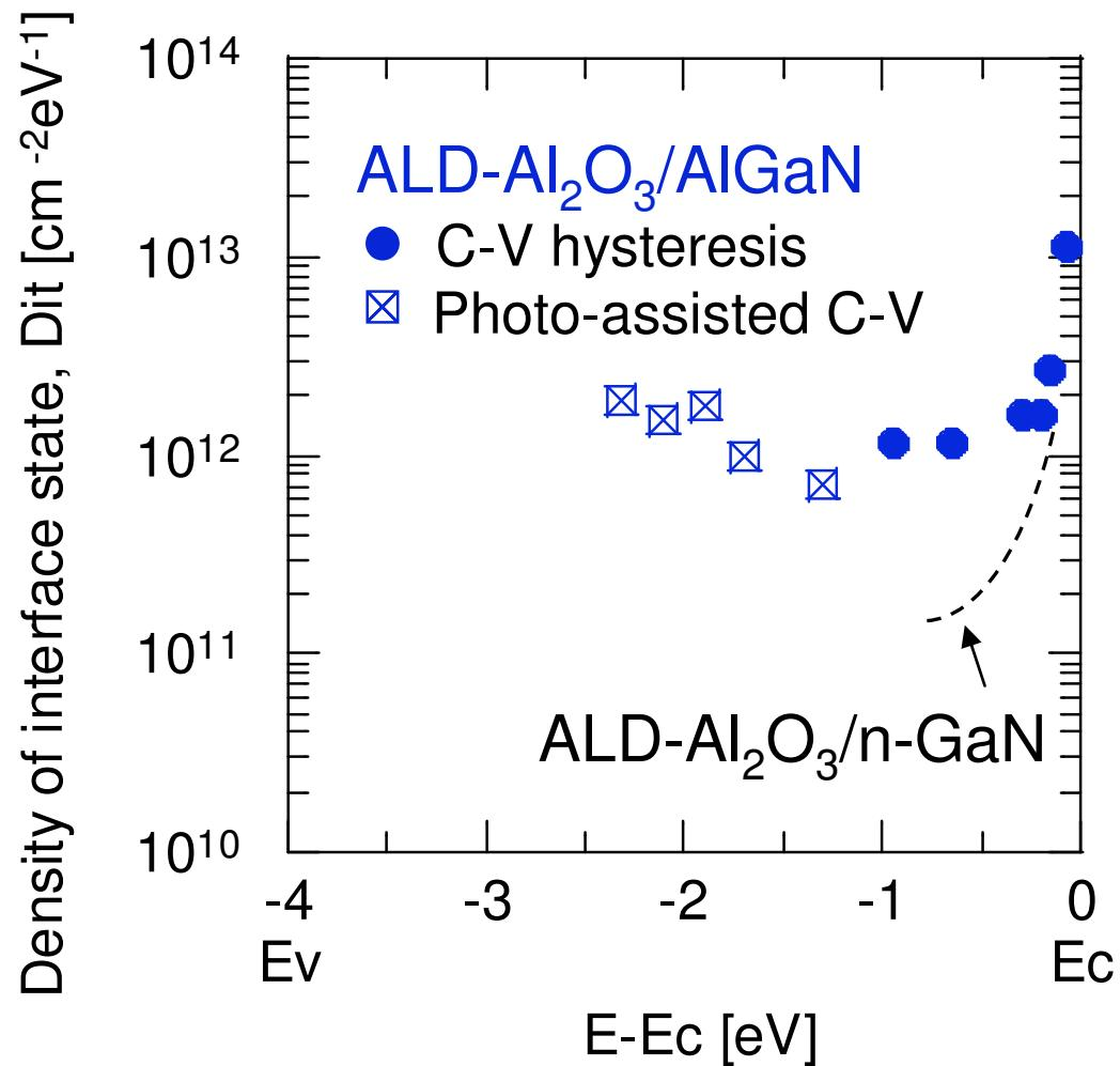
First report for the  $\text{Al}_2\text{O}_3/\text{AlGaN}$  interface using the HEMT-MOS structure
